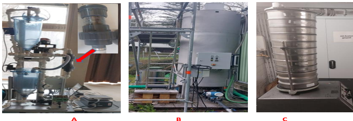
Fig. 1: A) Continuous Lab-scale GAC-Plant: used for the treatment of model wastewater and for finding related kinetics B) Continuous Large-scale GAC plant: used for application of the treatment technology in real wastewater C) Multi sieves apparatus: utilized for particle size distribution.
