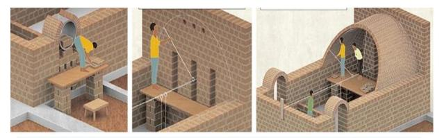
Fig8 . shows the Nubian vaults roofing structure in as a modern solution for rural Tanzania
