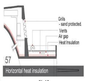
Fig12 shows horizontal heat insulation layers
