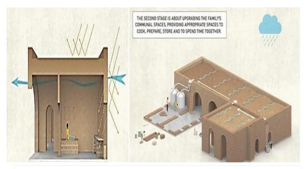
Fig7 shows roofing structure linned by rain collecting pipes and thick wall allow thermal insulation and cross natural ventilation
