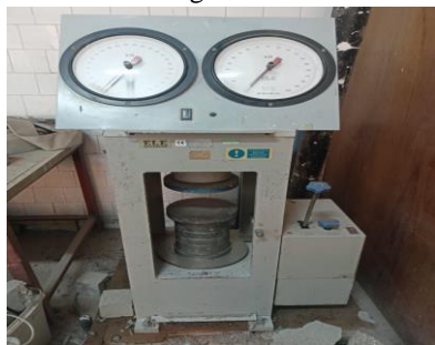
Fig. 4. Briquette Compressive Strength test machine
