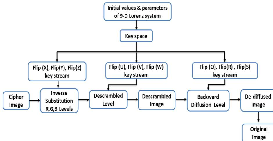
Figure 2: Framework of decryption algorithm
