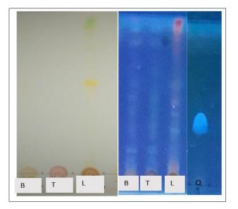
**Figure 7. Alkaloid chromatoplate**. Chromatographic condition: Stationary phase: Silica gel 60 F<sub>254</sub>. Mobile phase: toluene-ethyl acetate-diethylamine (35:10:5). *Legend: L: Leaves ; T: Stem Bark; B: Branch Bark.*
