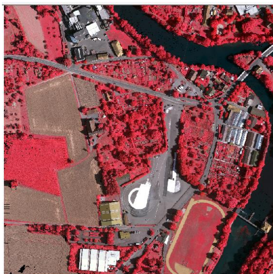
Fig. 1. An ortho image extracted from aerial imagery stereo pairs at rural landscape.
