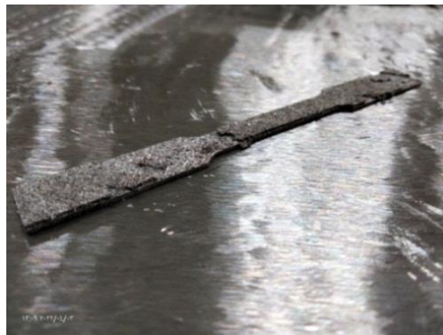
Fig. 4: Incompletely building at laser power 50 watts and scanning speed 200 mm/sec
