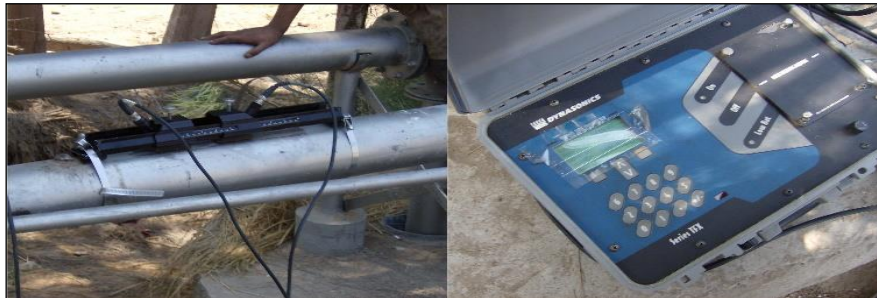
Fig. 2. Ultrasonic flow meter used to calibrate the improved Mesqas
