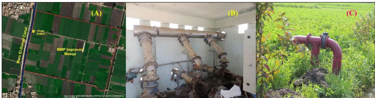
Fig. 7. The layout of second improved mesqa ( https://earth.google.com ) and photo of pumps and valves
