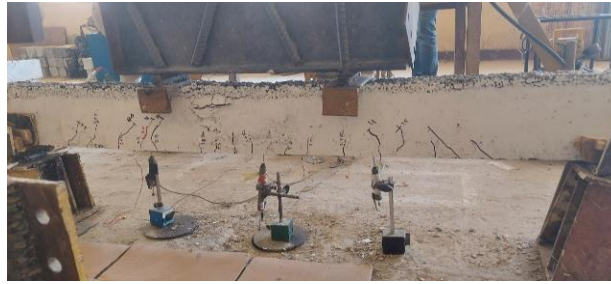
Fig. 10. Conducting the test on concrete beams and loading.
