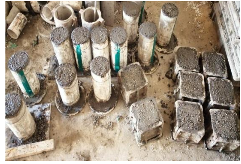
Fig. 4. Stage 2: Three lightweight concrete mixes
