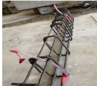
Fig. 8. Steel Strain Measurement
