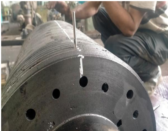
Figure 5. The roller during perforation longitudinal channels (Deshna factory).
