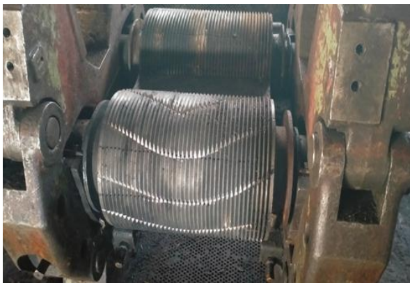
Figure 6. The modified rolls during mounting on mill (Deshna factory).
