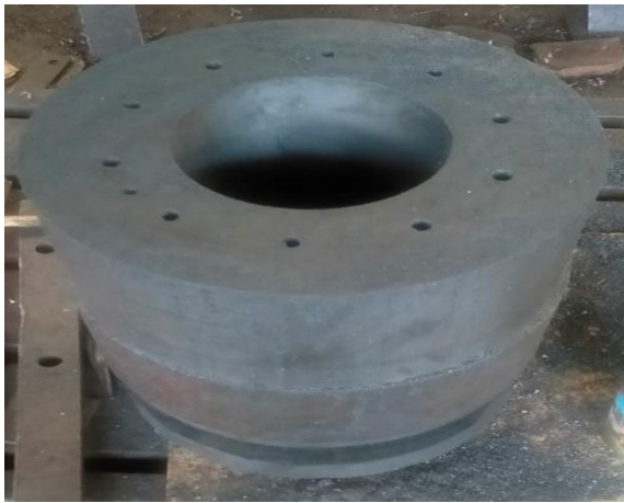
Figure 4. The shell after making a longitudinal hole (Deshna factory).
