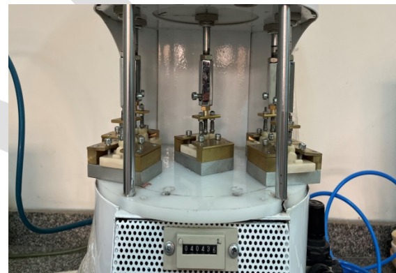
Figure 3. Cyclic loading of specimens.
