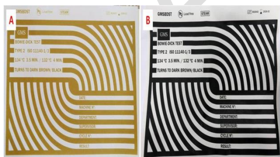
Figure 3: Show color change of Bowie dick test in successful sterilization cycle Color change to black. (A) Before sterilization (B) After sterilization.
