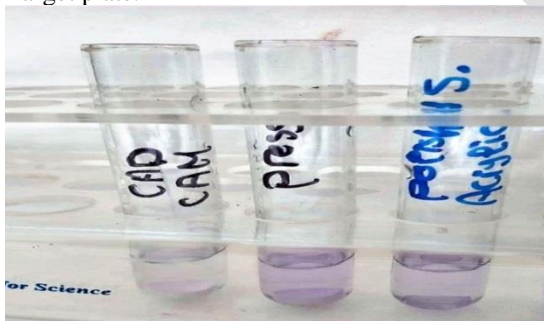
Fig. (5): Different acetic acid elusion colours owing to different stain uptake, corresponding to different amounts of biofilm formation.
