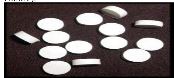
Fig. (1): Twelve milled BioHPP circular discs.
