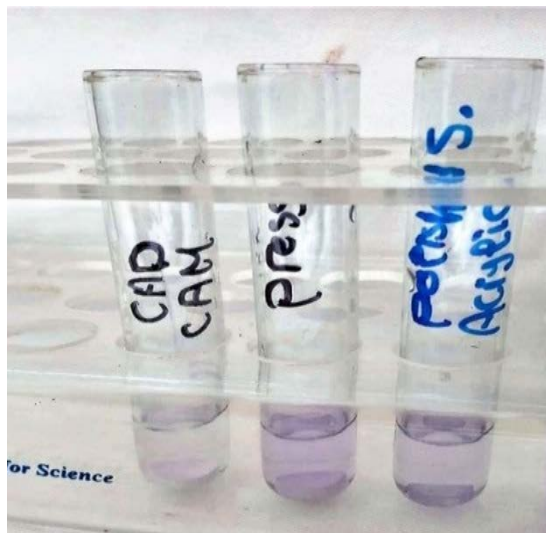
Fig. (5): Different acetic acid elution colours owing to different stain uptake, corresponding to different amounts of biofilm formation.
