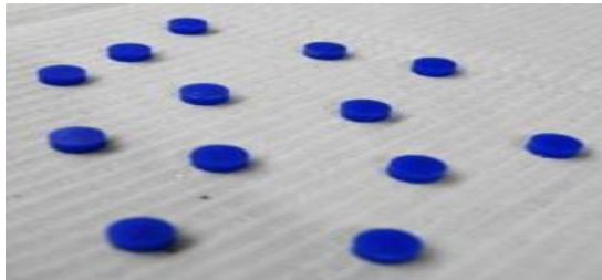
Fig. (3): Milled circular wax discs from KATANA wax blanks.
