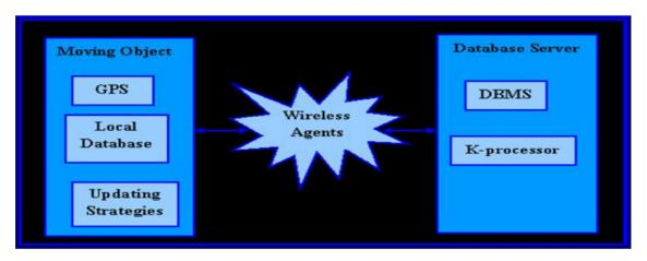
Figure 1. Architecture of the MOD updating system
