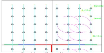
Figure 3. layout of fixed sprinkler system networ
