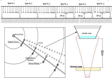
Fig. 6. The location of catch cans under center pivot systems
