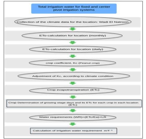
Figure 4. Process planned of method for calculating the irrigation requirements of peanut crop
