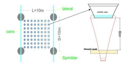
Figure 5. Layout the sprinklers in the field to test the uniformity for fixed irrigation system
