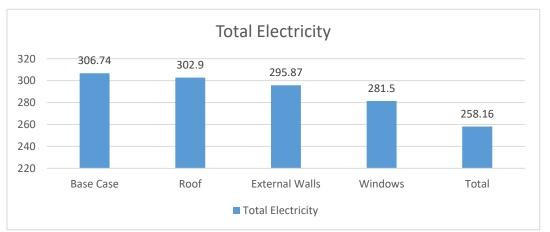
The results of adding VIPs to the external wall insulation and TiO2 Cladding showed that total energy use was reduced by more than 3.5%. the adding VIPs to the roof reduce about 1.37%.
