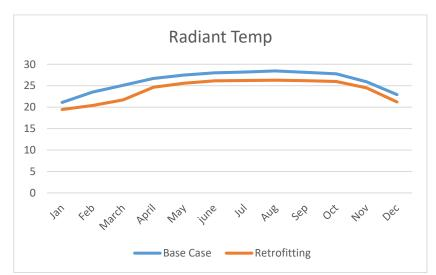
Radiant Temp = The highest radiant temperature recorded was  $28.45^{\circ}$ C which, in turn, decreased by  $2.14^{\circ}$ C.
