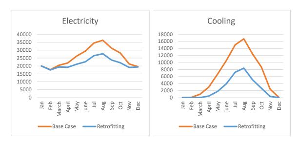
Total Electricity = 258.16 MWh Before = 306.74 MWh Decrease = 16%
