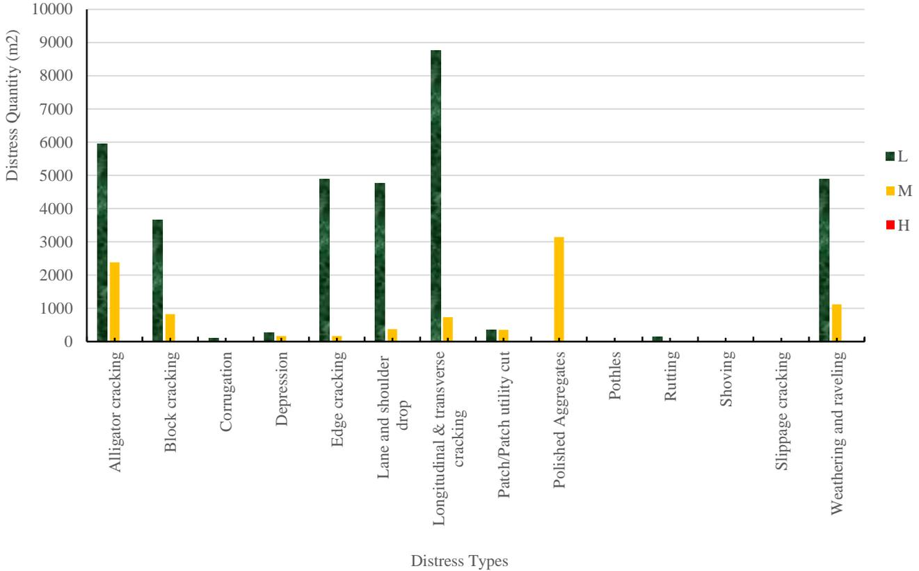
Fig. 7 Distress types and their quantity in section 2.
