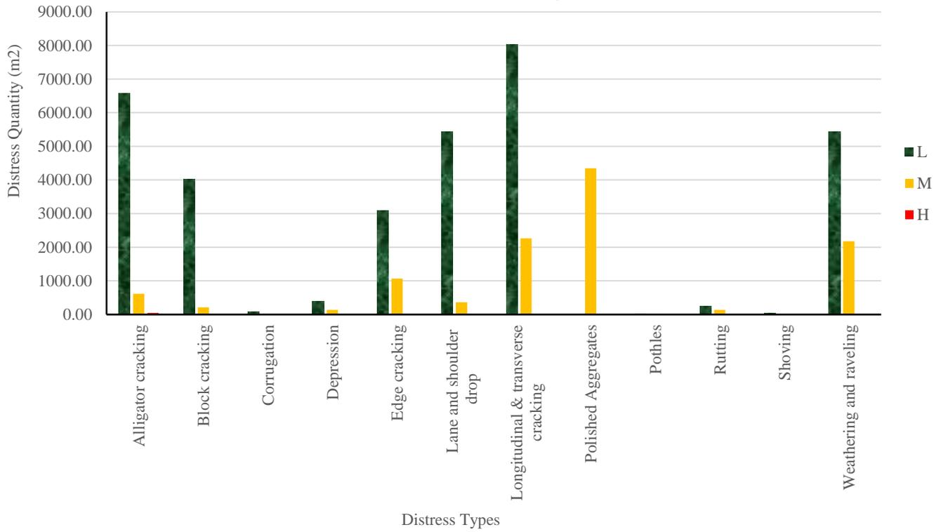
Fig. 8 Distress types and their quantity in section 1.
