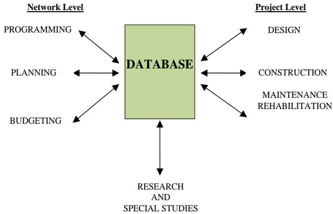
Fig. 1. The Main Components of a Pavement Management System [4].
