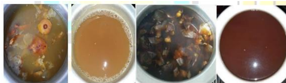
Figure 10: Extraction of Mordant from Pomegranate and Onion peel
