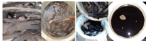
Figure 9: Teak wood dye Extraction Process
