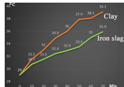
Figure (10): Time lag for clay bricks with Recycled Iron slag bricks
