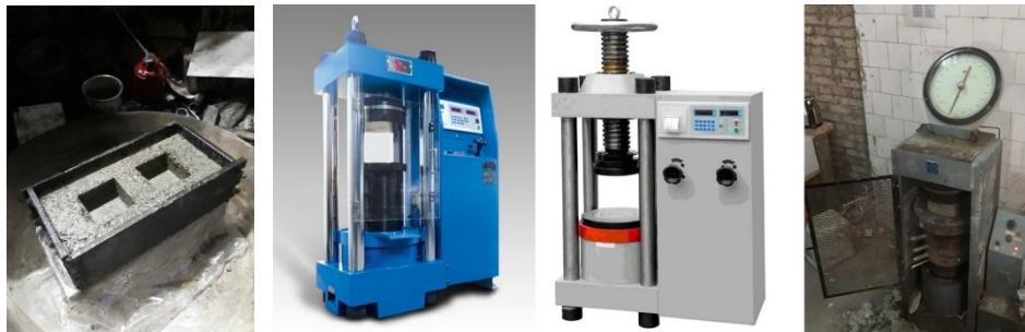
Figure 2: Different types of compression testing machines and a sample of testing bricks in its iron form [11]
