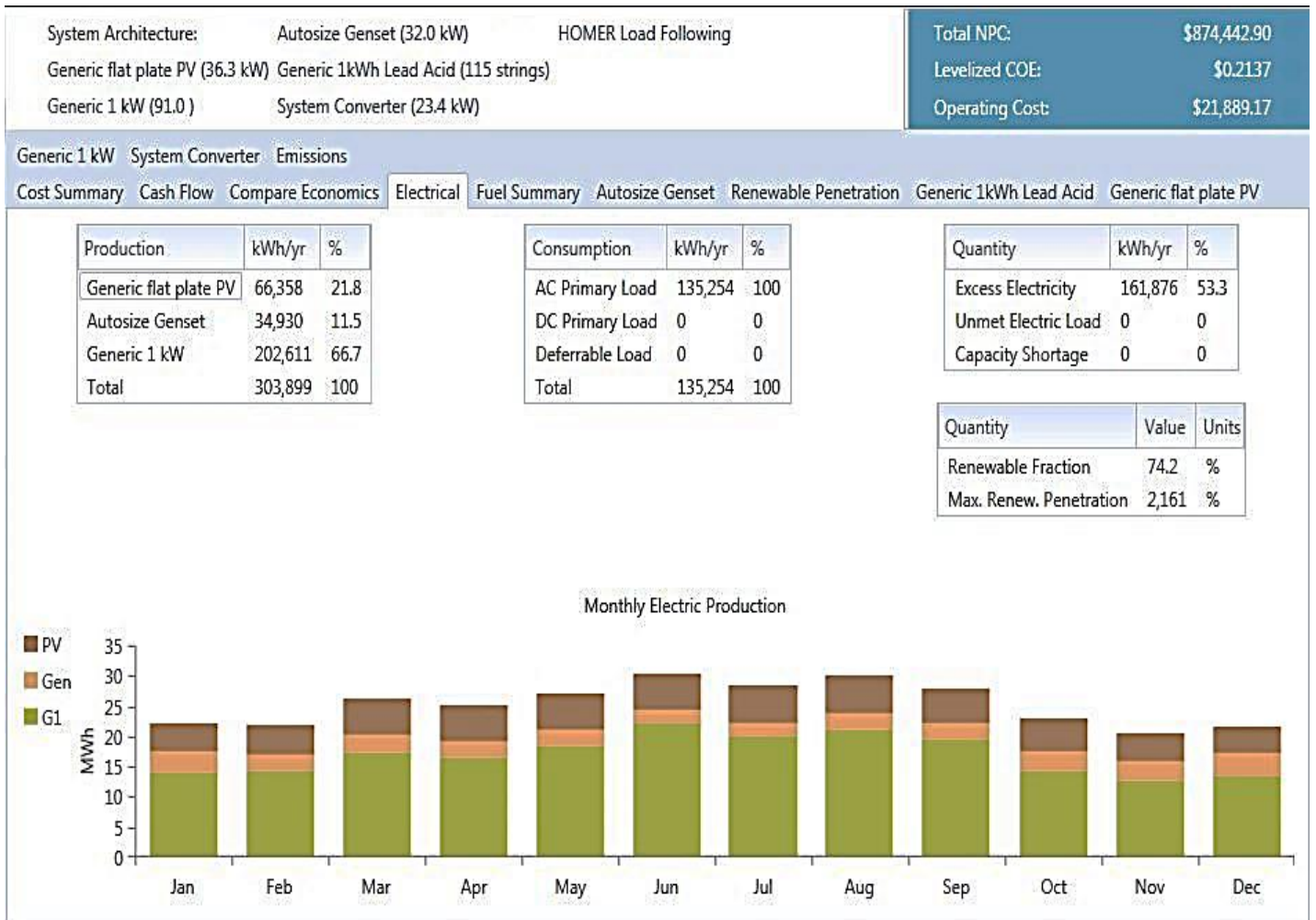
Fig. 16. Electrical Production Summary for HRES without DSM in Qena governorate
