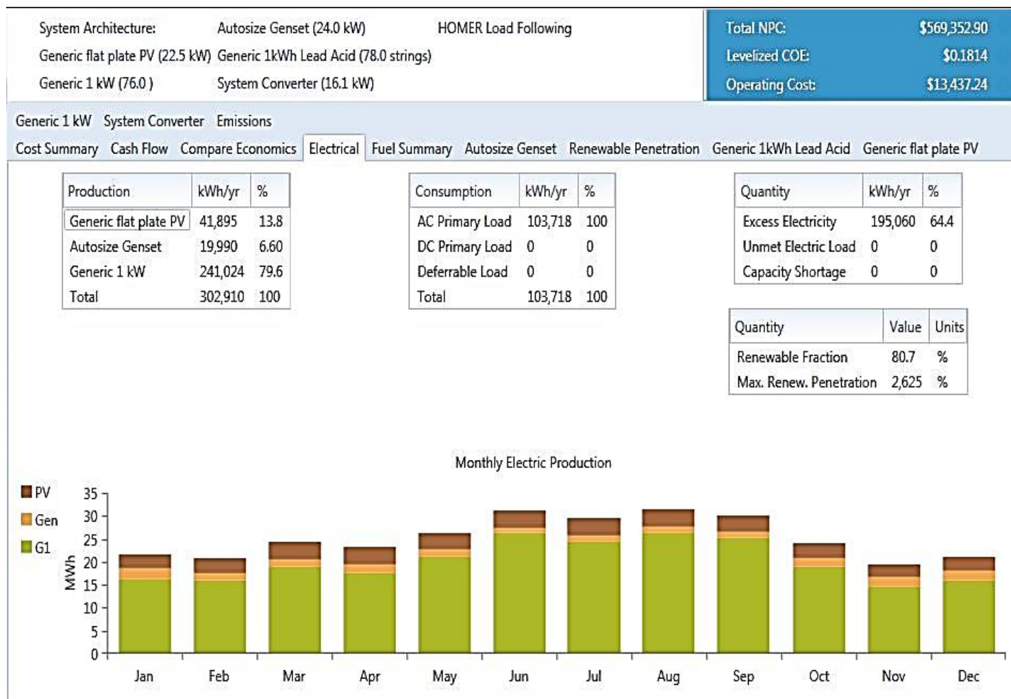
Fig. 21. Electrical Production Summary for HRES with DSM in Red Sea governorate
