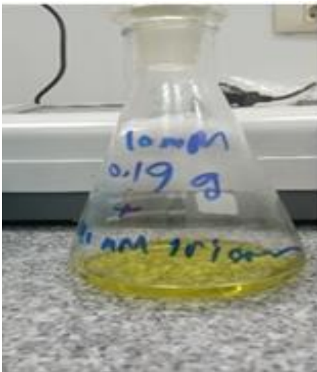
Figure 2. Preparation of AuNPs by a chemical reduction method.
