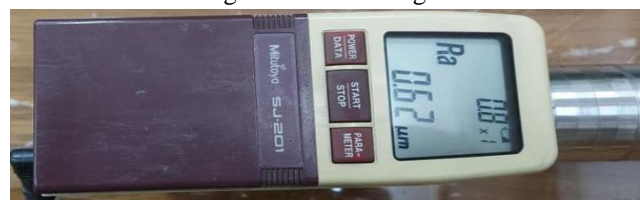
Fig 7. Surface roughness measurements for the burnished workpiece using sj-310 Mitutoyo surfest.
