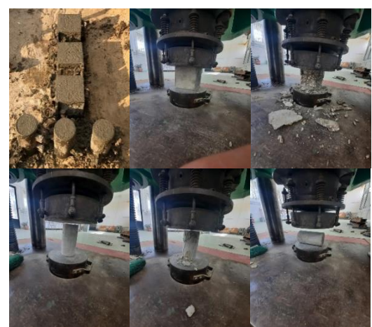
Fig. 4. Testing and pouring concrete for cubes and cylinder specimens
