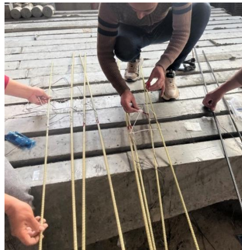
Figure 6- Setting the strain gauge on bars.
