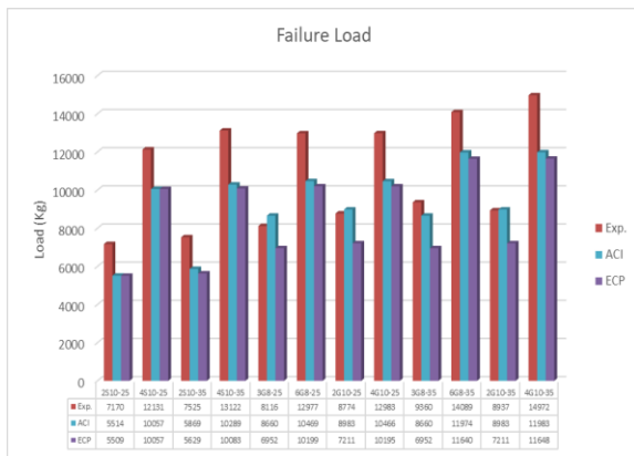
Figure 22- Comparison between experimental and analytical failure loads for different tested beams.
