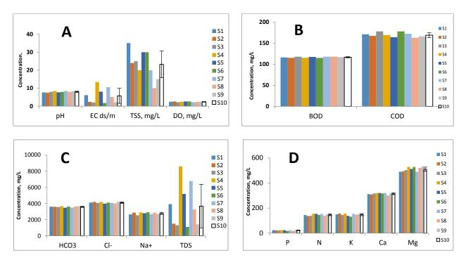
Figure 6. Results of the physicochemical parameters of the Hemodialysis Wastewater samples analyzed
