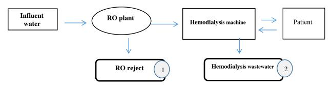
Figure 2. A diagram of the wastewater produced by hemodialysis and the RO treatment process.
