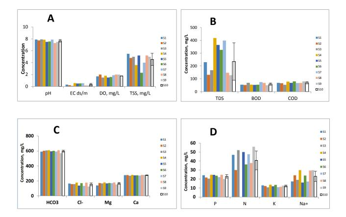
Figure 4. Results of the physicochemical parameters of (RO) reject samples analyzed S 10.
