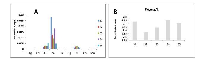
Figure 5. Heavy Metal Concentrations in the RO reject water samples analyzed.
