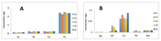
Figure 7. Heavy Metal Concentrations in Samples from Hemodialysis Wastewater
