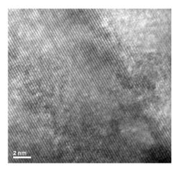
Figure 3 exhibits a HRTEM from another LED on a QW area, with the In-clustering seen clearly. These nano-structural or QDs features are closely correlated with results from HRXRD, PL/PLE. Figure 4 shows a XRD pattern for an InGaN MQW with 8-QWs, with multiple narrow satellite bands.
