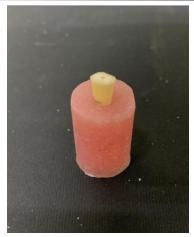
Figure 1. Photograph showing root mounted in self- cure acrylic resin block.
