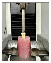
**Figure 2.** Photograph showing a tooth mounted in acrylic resin after being fractured using universal testing machine.
