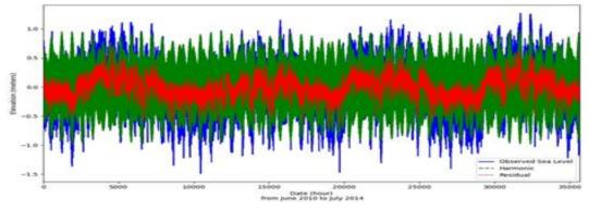
**Fig. 6.** Observed – harmonic - residual from harmonic analysis from June 2010 to July 2014
