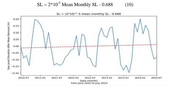
Fig. 5. Monthly fluctuations in sea level at PT for the duration of the study
