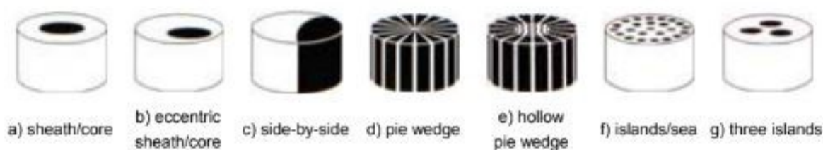
Figure 2: Typical bicomponent fibre type
