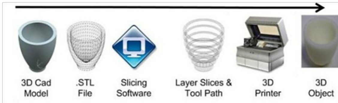
Fig .1: The stages of the 3D printing process [1]
