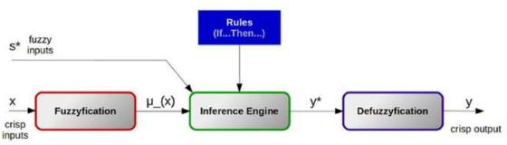
Figure 3: Fuzzy control system diagram [51]
