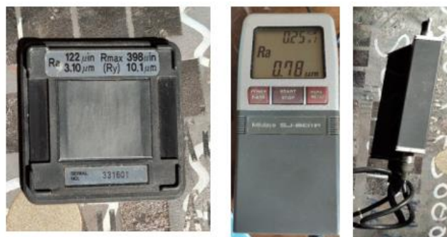
Fig 4. Set up for surface roughness measurement tester
