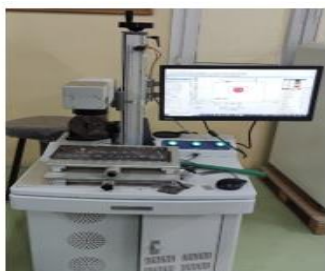
Fig 1. 3D Laser engraving machine used for the experiments
