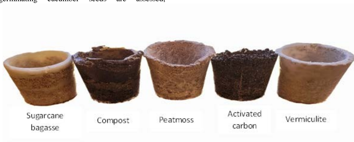
Fig. (1): Biodegradable cultivating pots fabricated from a neat type of filler
