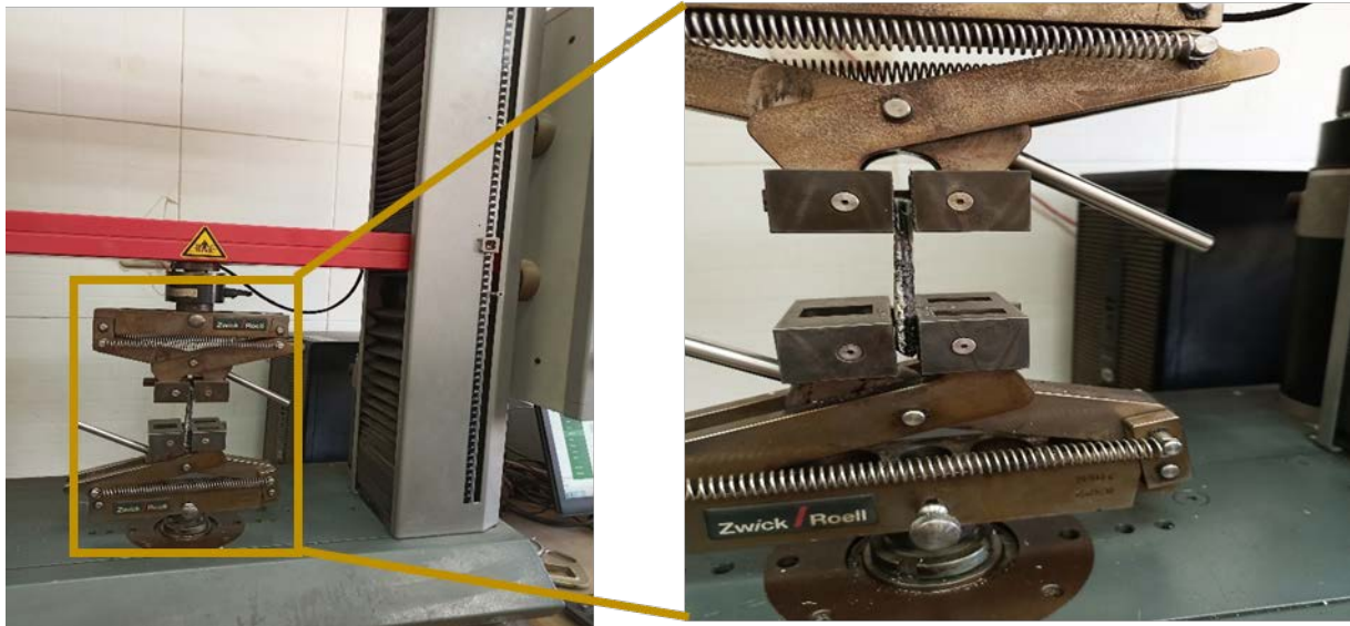
Fig. (2): Tensile strength measurement of the samples.
