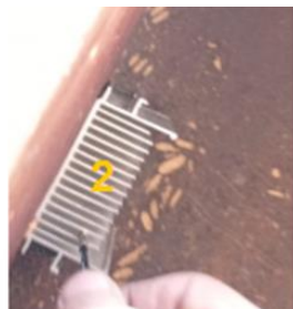
2- Aluminum heat sink's fins
