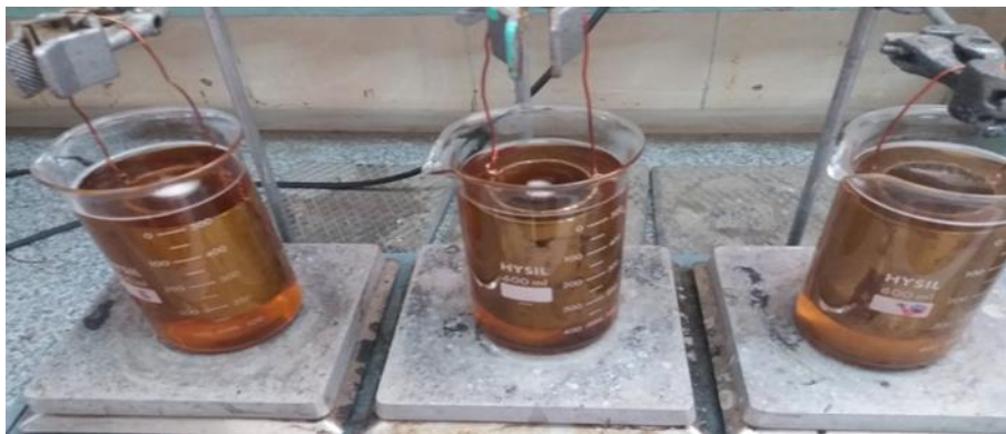
Figure 4: Cleaning of the evaporator tubes with scales
