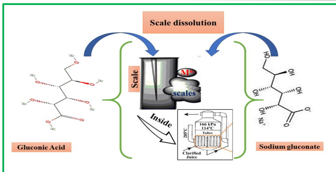
Figure 11: Mechanism for scale dissolution by organic acids
