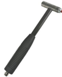
Figure 4. Impact Hammer Model PCB-086C-03.
