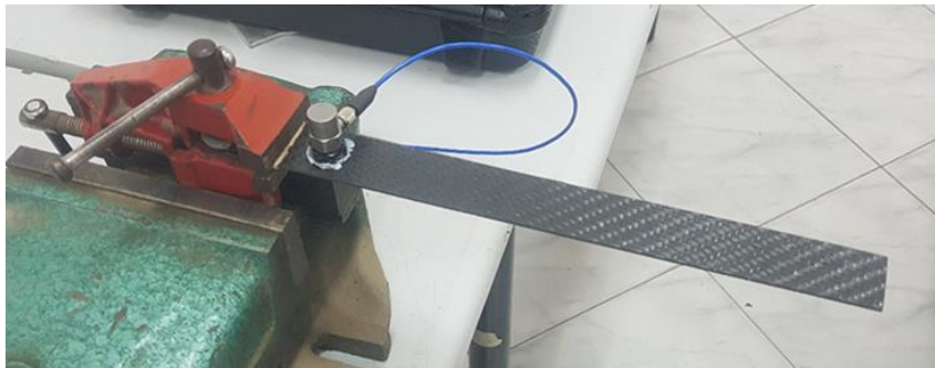
Figure 5. Beam fixation and accelerometer location.
