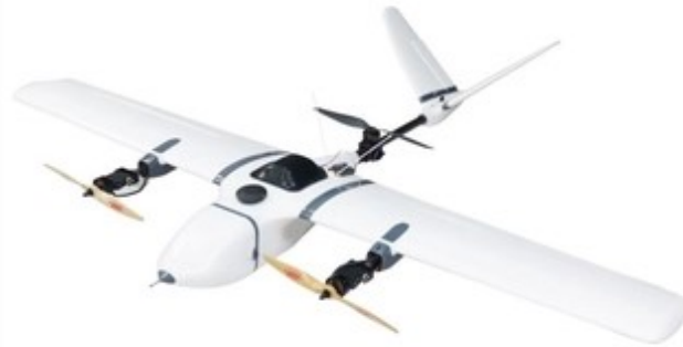
Figure 2. Nimbus 1800 Tilt-rotor UAV.
