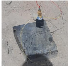
Figure 3. Perforator charge attached to steel target.
