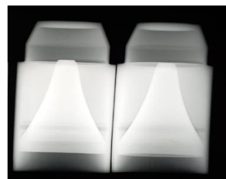
Figure 2. A sample of the X-ray photograph of a perforator charge.
