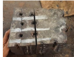
Figure 4. Cutting of laminated layers of 1006 steel target after tests.
