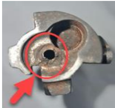
Figure 6. Close-up of a fractured bolt.
