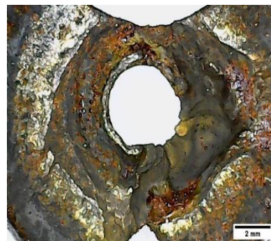
Figure 9. A clear visual inspection of the failed bolt surface.
