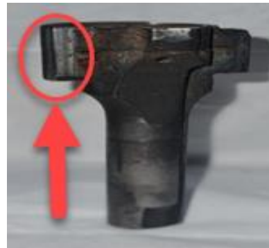
Figure 7. Failed bolt with worn lugs.
