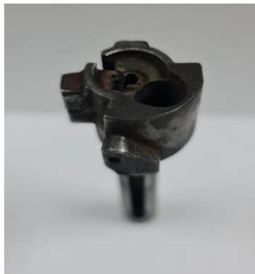
Figure 3. Failed bolt body.
