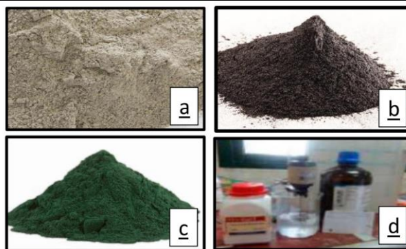
Fig. 1. The images of materials used in this study: (a) soil, (b) Fly ash, (c) Polyaniline, and (d) sodium silicate & sodium hydroxide solution.
