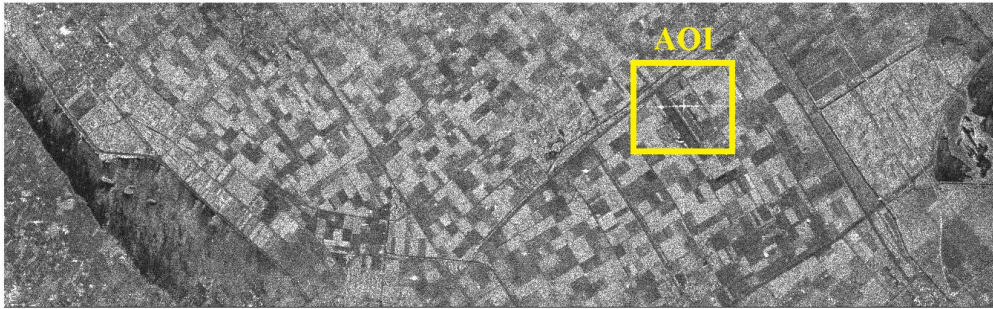
Figure 7. Focused image of ERS satellite produced by the Range Doppler Algorithm (RDA).
