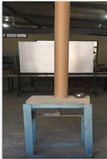
Figure 4. Preparation of drop weight impact test.
