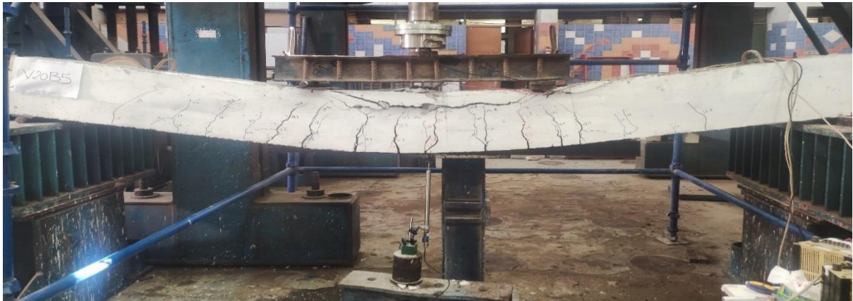
Figure 6. The Concrete Slippage in V20B5
