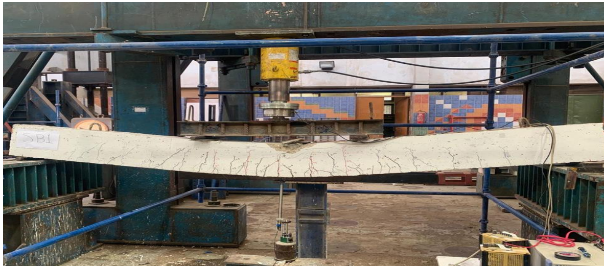
Figure 7. The Failure in SB1
