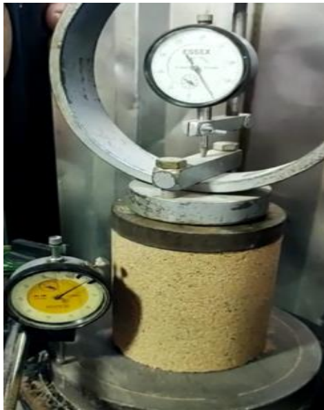
Figure 9 Specimen with 20% solution of SS21, during test.
