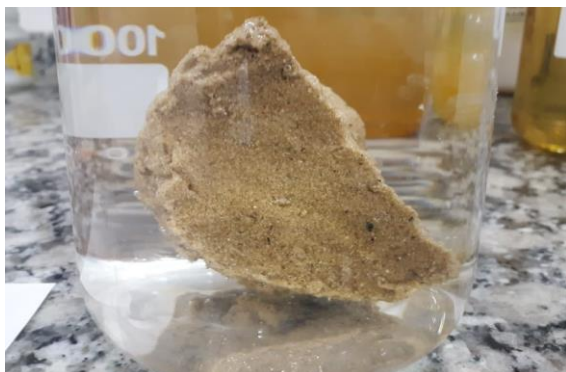
Figure 13 Fragment of sand stabilized with SS21. That sample is still under water, and at the moment is 1 year and counting. This is the live proof of the potentialities of SS21 for waterproofing and the justification for unsoaked condition approach. The specimen has a 20% of OMC replacement with SS21.
