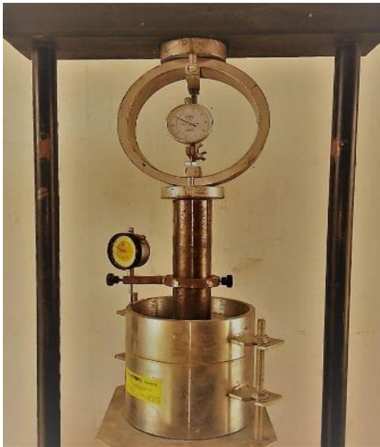
Figure 11 Standard arrangement from WEG for CBR test showed on previous paper (16).
