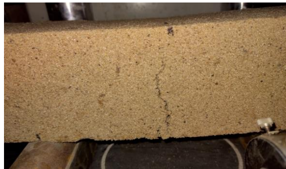
Figure 17 Beam on failure during test. 30% of SS21.
