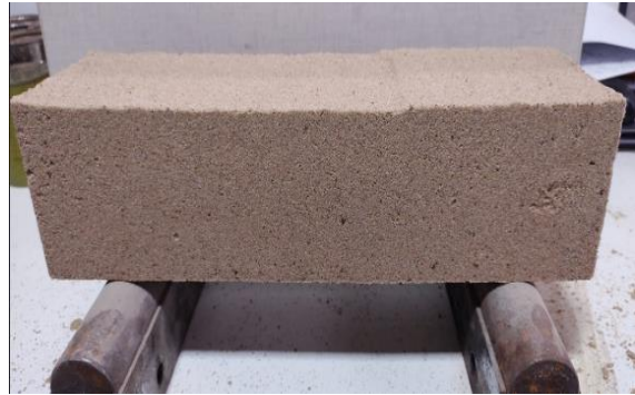
Figure 16 100x100x350mm beam of sand with 30% of SS21.
