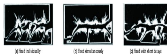
Figure 14 Effects of using delays on presplit holes [51]
