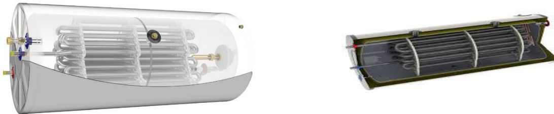
Fig. (4) Schematic representation of the Heat Exchanger inside the hot storage tank
