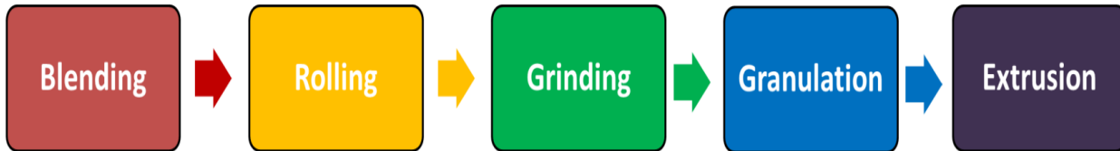
Fig. 3: Schematic for solventless extrusion process for manufacture of MDB propellant
