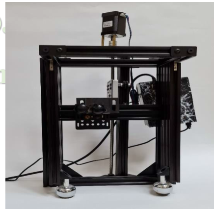
Figure (1) photograph showing the dynamic cyclic fatigue testing device
