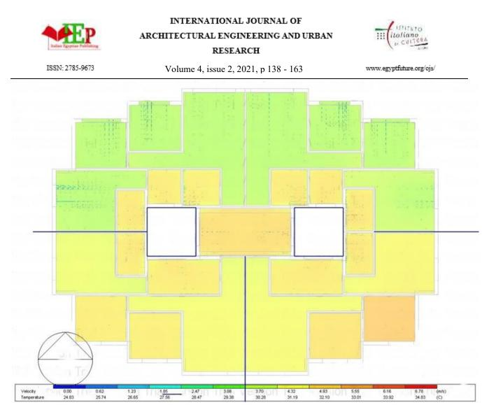
Figure 10 Simulation results for the indoor air temperature and velocity vectors for the Ground Floor Plan,
