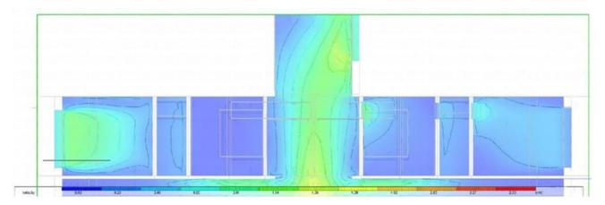
Figure 19 CFD slice showing the Velocity contours direction in longitudinal section 1
