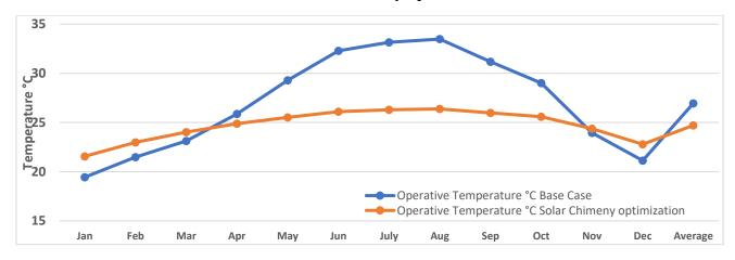
Figure 22 Comparison of Operative air temperature for Typical Floor Plan (3rd floor) of the base case and solar chimney optimization, source: the researcher.
