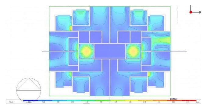
Figure 16 CFD slices showing the air velocity pattern of Typical Floor Plan (3rd floor) on using solar chimney showing the best and highest airflow circulation
