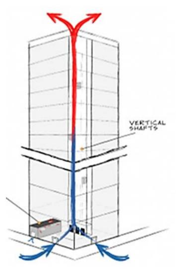
Figure 4 A Diagram illustrating Stack Effect [8]
