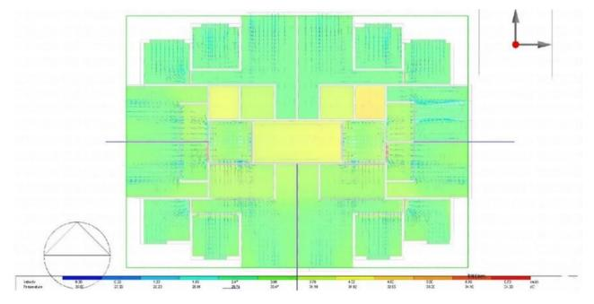
Figure 17 CFD slices showing the operative temperature and the air velocity pattern of the Typical Floor Plan (3rd floor) using solar chimney
