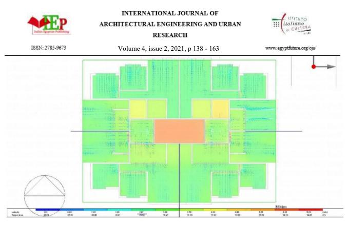
Figure 20 CFD slices showing the operative temperature and the air velocity pattern of the Last Floor Plan: (5th floor) plan on using solar chimney
