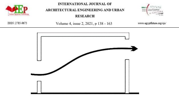
Figure 2 Staggered openings in vertical level [3]
