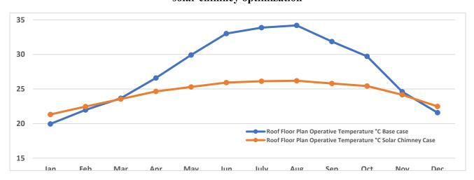
Figure 21 Comparison of Operative air temperature for Last Floor Plan: (5th floor) of the base case and solar chimney optimization.
