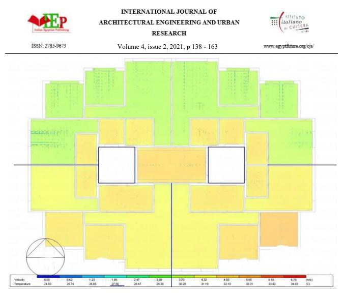
Figure 11 Simulation results for the indoor air temperature and velocity for the Typical Floor Plan (3rd floor),
