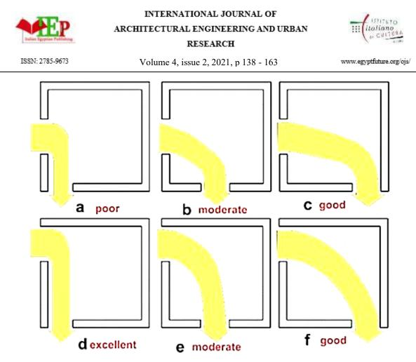
Figure 1 Adjacent openings configurations [2]
