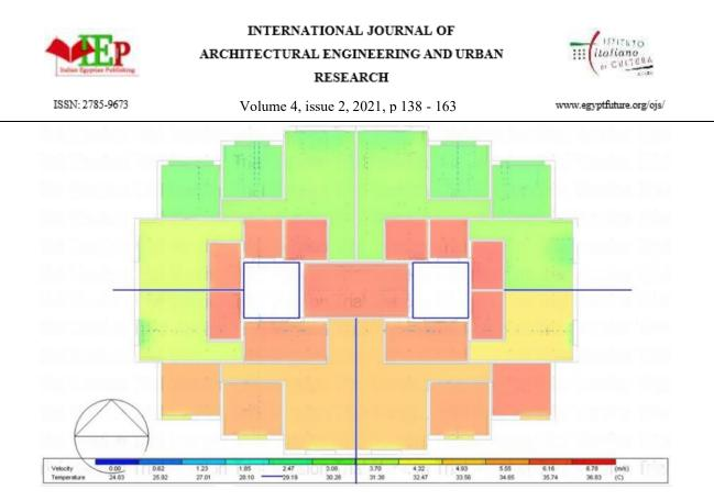
Figure 12 Simulation results for the indoor air temperature and velocity vectors for the Last Floor Plan: (5th floor
