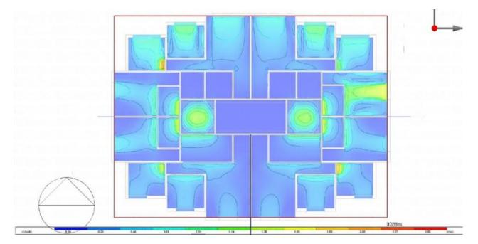
Figure 21 CFD slices showing the air velocity pattern of the Last Floor Plan: (5th floor) on using solar chimney showing the best and highest airflow circulation
