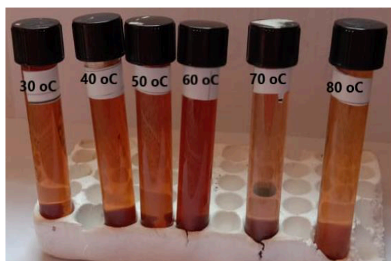
Figure 9. Effect of different temperatures (30 °C- 80 °C) on ULAgNPs synthesis in a reaction solution containing 5:5, v/v ratio of 4mM AgNO 3 and algal extract.
