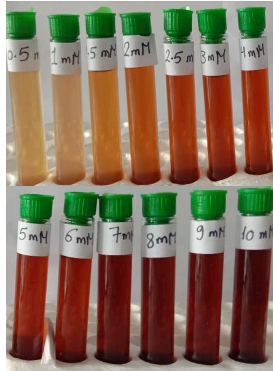
Figure 7. Effect of different concentrations of \text{AgNO}_3 (in mM) on ULAgNPs biosynthesis containing 5:5, v/v ratio at static conditions and 30 °C for 48 h.
